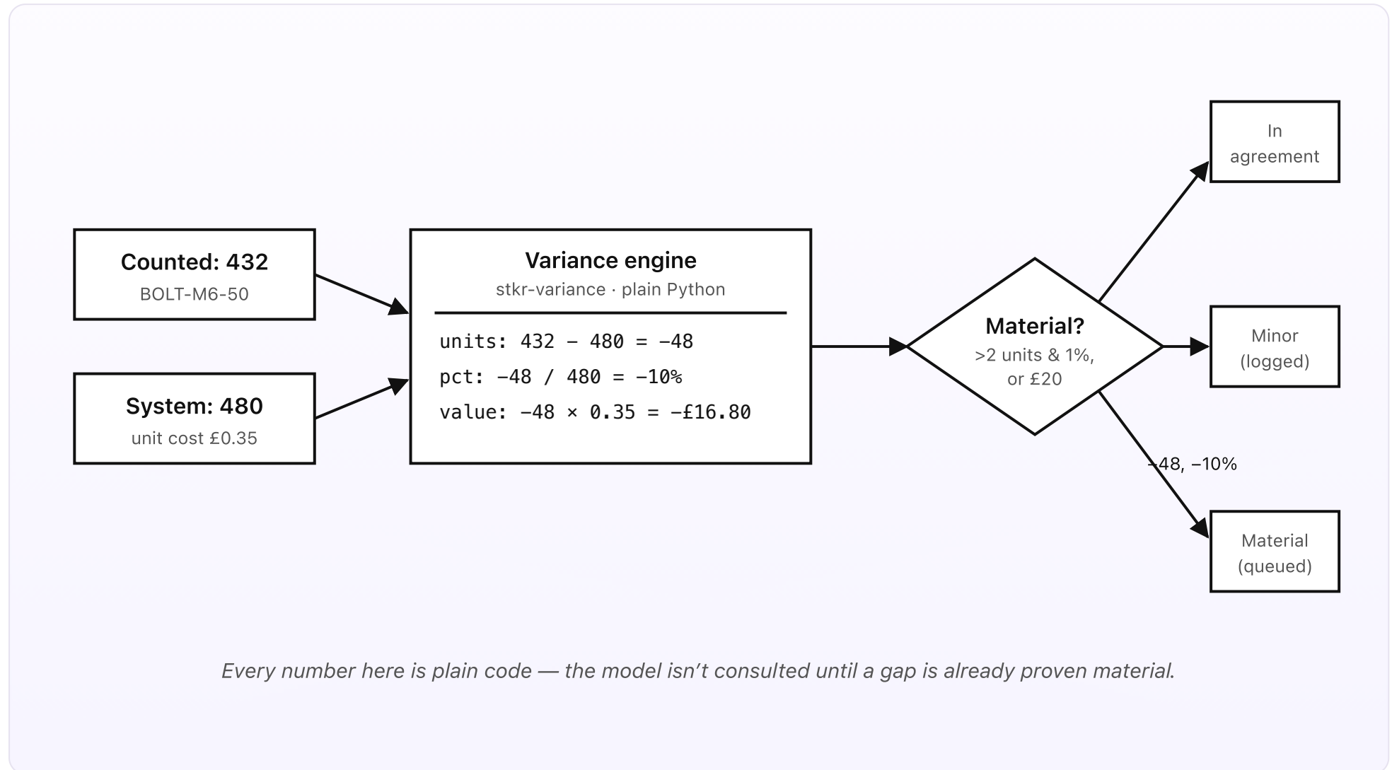
Fig 3. One line through the engine. Counted 432 against a system 480 gives -48 units, -10%, and -£16.80. That clears both the unit and the percent thresholds, so the line is a material variance and goes on to cause suggestion. A line inside tolerance would be logged and left.
